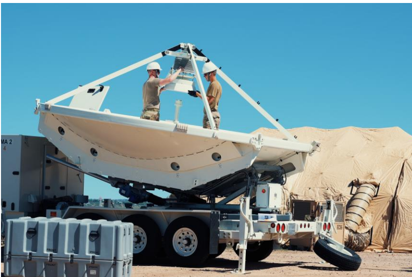
Guardians and airmen assemble a satellite communications dish at Peterson Space Force Base. Source: DVIDS
